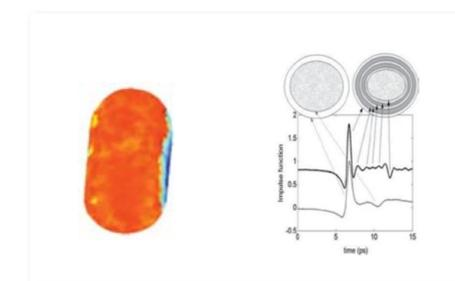
Figure 3: False-color 3D THz pulsed image (a) of enteric coating tablet determined from the THz time-domain waveform (b) of the tablet (courtesy of TeraView, Cambridge, UK).
