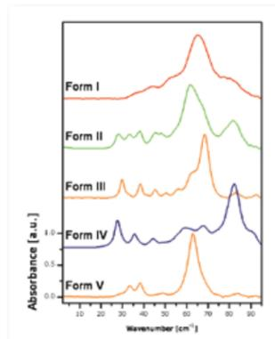
Figure 1: THz spectra of sulfathiazole polymorphic forms. Spectral features relate to intermolecular interactions. (Spectra offset for clarity, courtesy of TeraView, Cambridge, UK).
