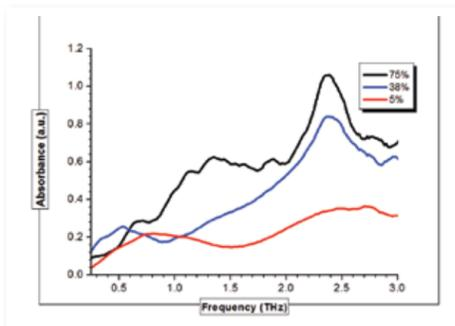
Figure 2: THz spectra of semi-crystalline polymers, showing changing spectra with increasing crystallinity.
